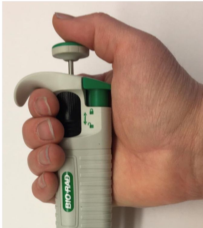
Figure 2: How to hold a micropipette. Your thumb should rest on the plunger and your other fingers should wrap around the barrel.
